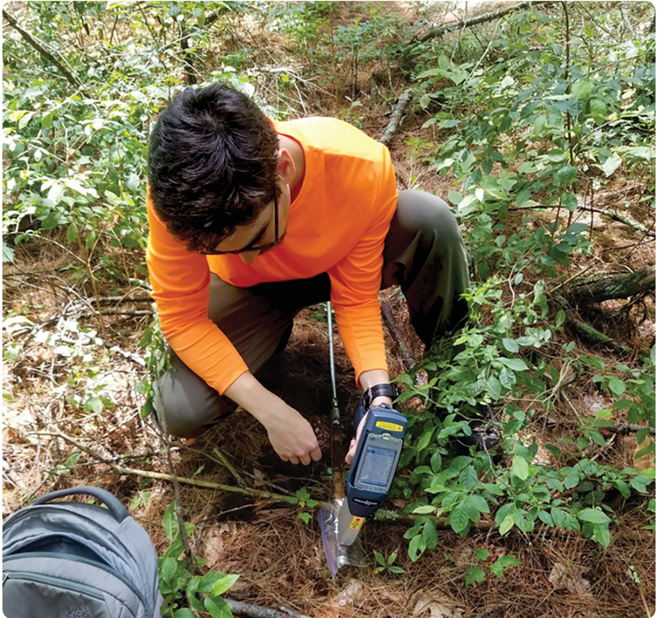
First author Mark Higgins measuring arsenic and lead levels in soils at depth using an X-ray fluorescence device and soil probe. Photo courtesy of Meredith Metcalf.
