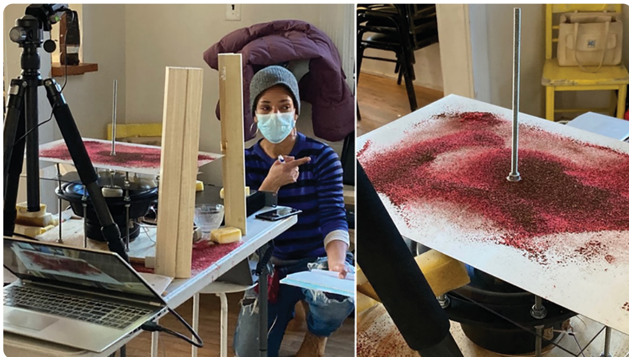
(Figure 1) Left: Candy Schibli at the cymatic rig. Right: Close-up of the vibrating metal plate with the ground coffee-sand mixture. The results of this work were presented at a Coffee Science Foundation poster session in Boston at the Specialty Coffee Expo in April 2022. For more information, see www.southeasternroastery.com/research .
