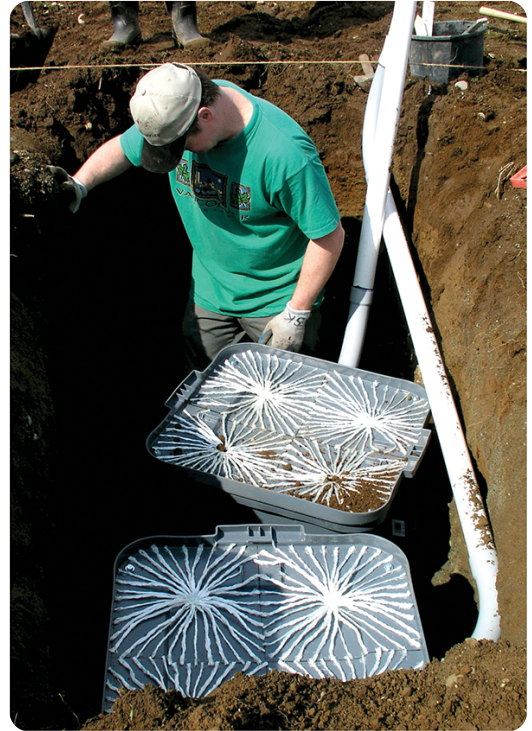
Scientist Tom Forge installs passive capillary wick samplers at the bottom of the rootzone prior to planting raspberry rows for the team’s multi-year experiment. The researchers dug 32 such holes to hold the instrumentation, which measured nitrate levels in water captured beneath the plants and the alleys. Photo by Shawn Kuchta.
