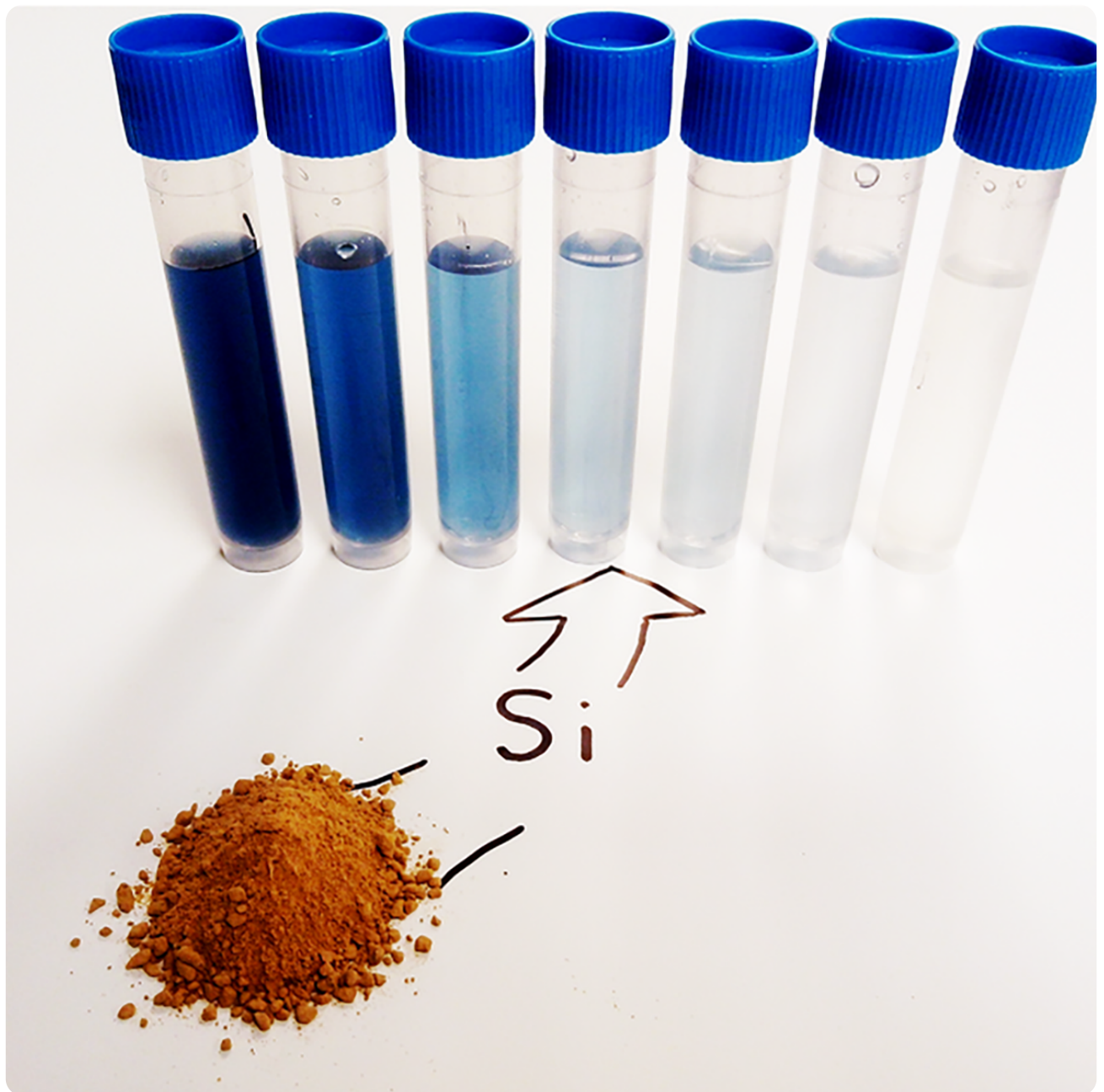
Color development due to increasing Si concentrations in the molybdate blue method for analyzing monomeric silicic acid. Photo courtesy of Matt Limmer.
