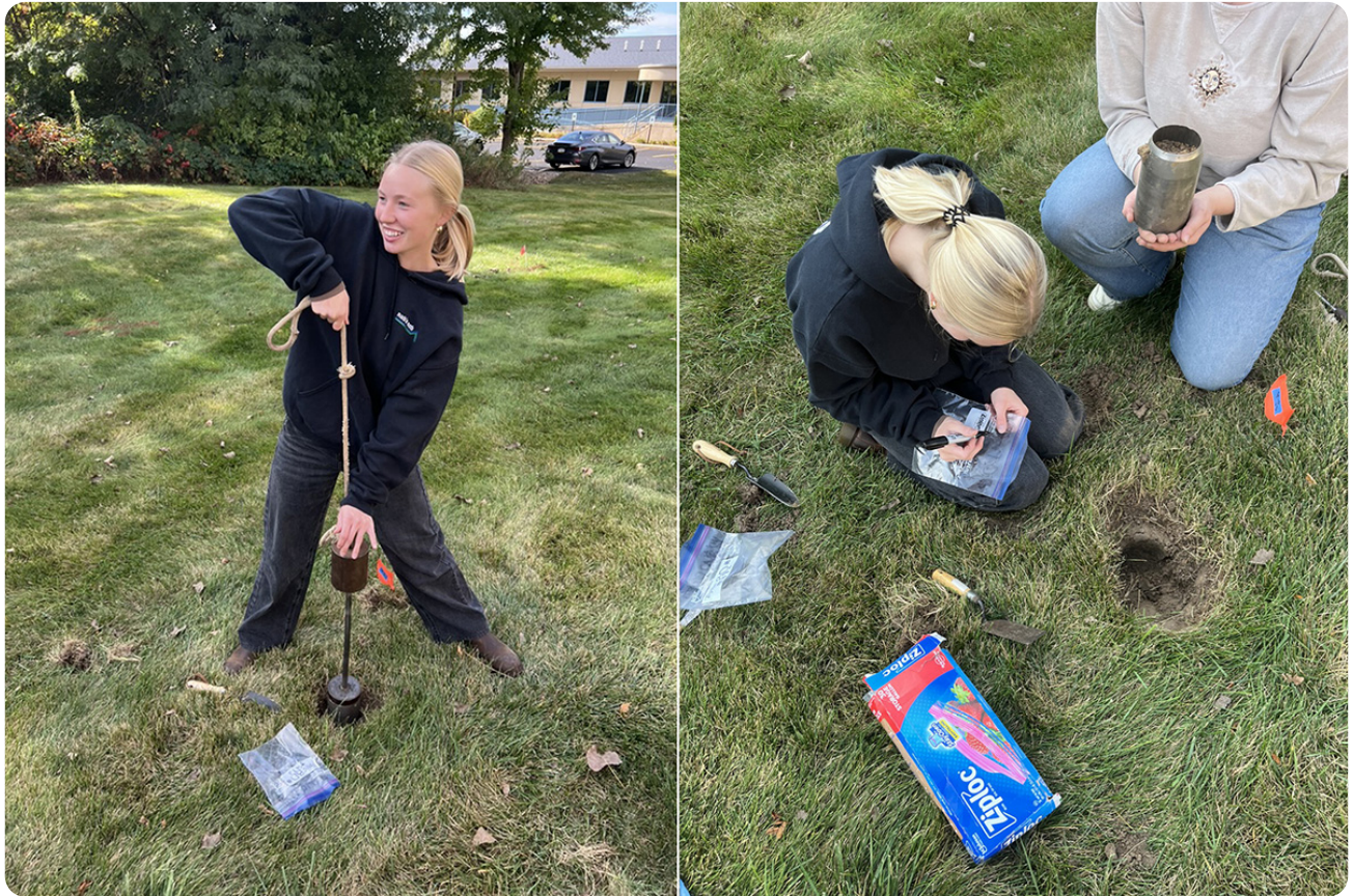
Cammy Whitcomb gathers soil for bulk density analysis. Photos courtesy of Lexie Hedrick (left) and Megan Zlimen (right).
