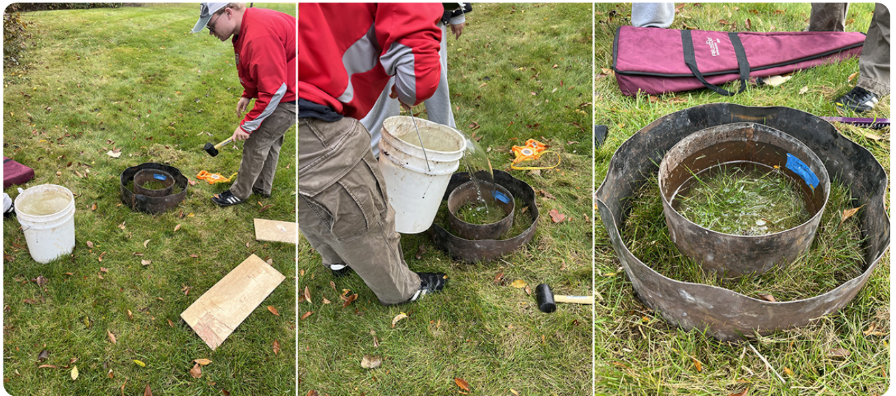
Rings standardize the amount of water poured during an infiltration test. Owen Weisse then times how long it takes for the water to drain through the soil. Photos courtesy of Megan Zlimen.
