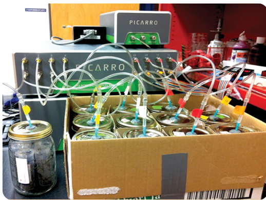
Figure 1, Standardized microbial respiration. Mason jars filled with soil samples are connected with needles to a Picarro Isotopic Gas Chromatography Machine to measure carbon dioxide release following rewetting of sieved, air dried soil.
