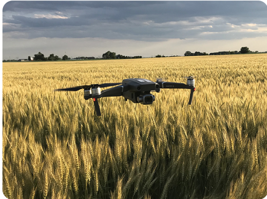
Multirotor drone with an RGB camera. Photo courtesy of Photo by Brad Bernhard.
