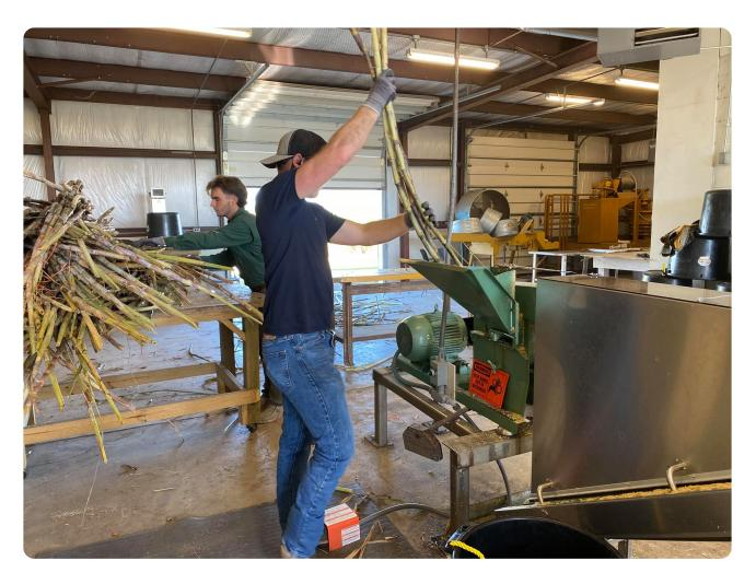
Blanchard passes whole sugarcane stalk samples through a shredder so the samples can be analyzed for sucrose content traits. Photo courtesy of Brayden Blanchard.
