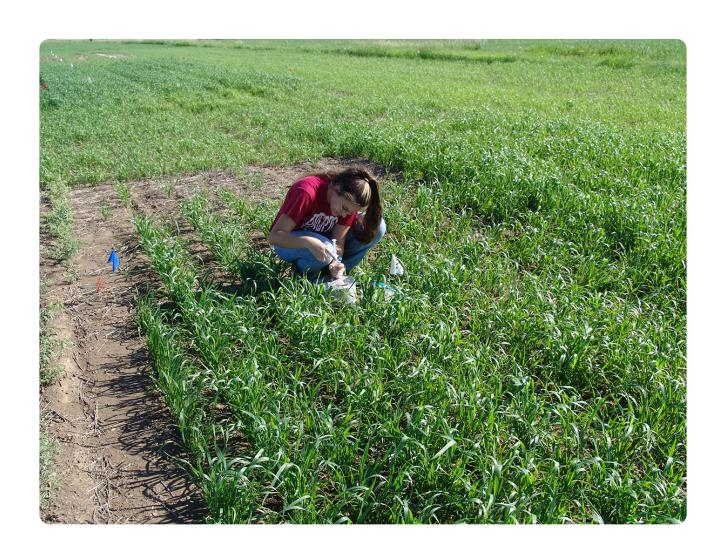
Greenhouse gas sampling under dryland spring wheat using a static chamber. Photo by Upendra Sainju.
