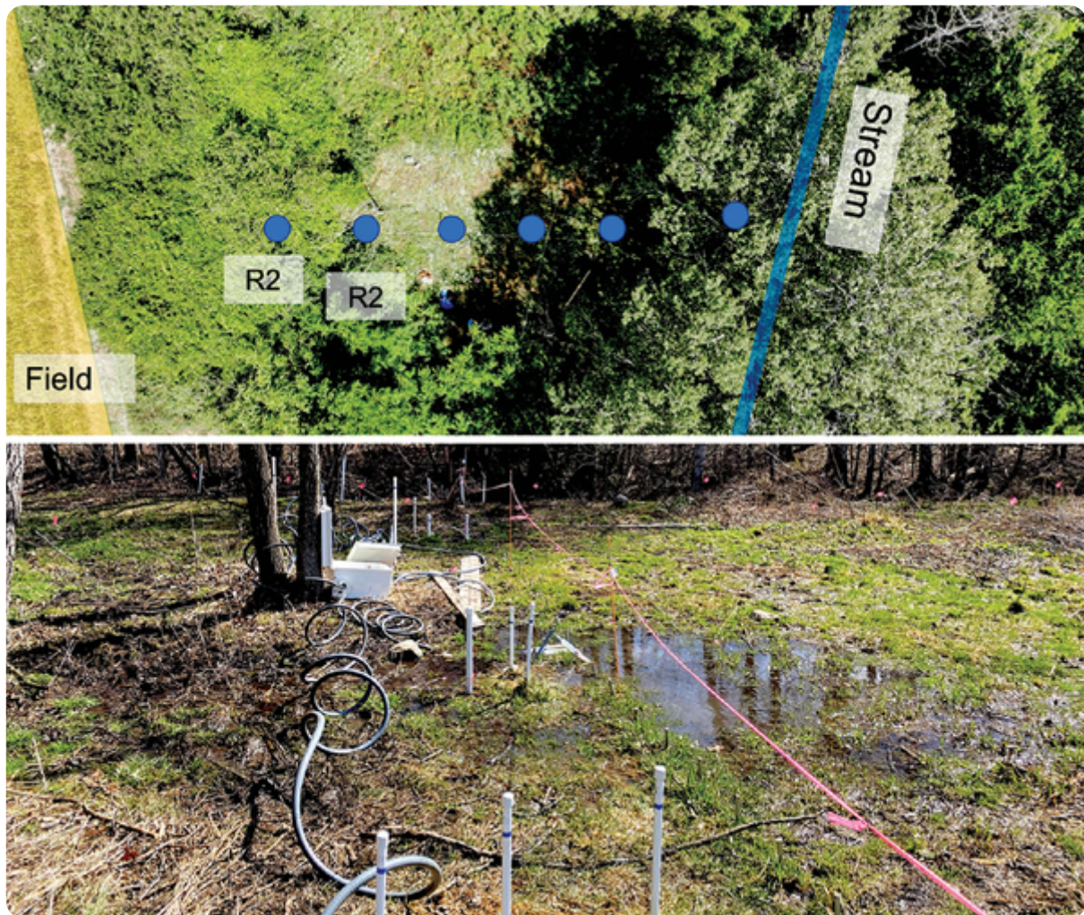
Top: Aerial image of a monitoring transect between an agricultural field and stream to examine the fate of phosphorus in the subsurface of a riparian zone. Bottom: Field
