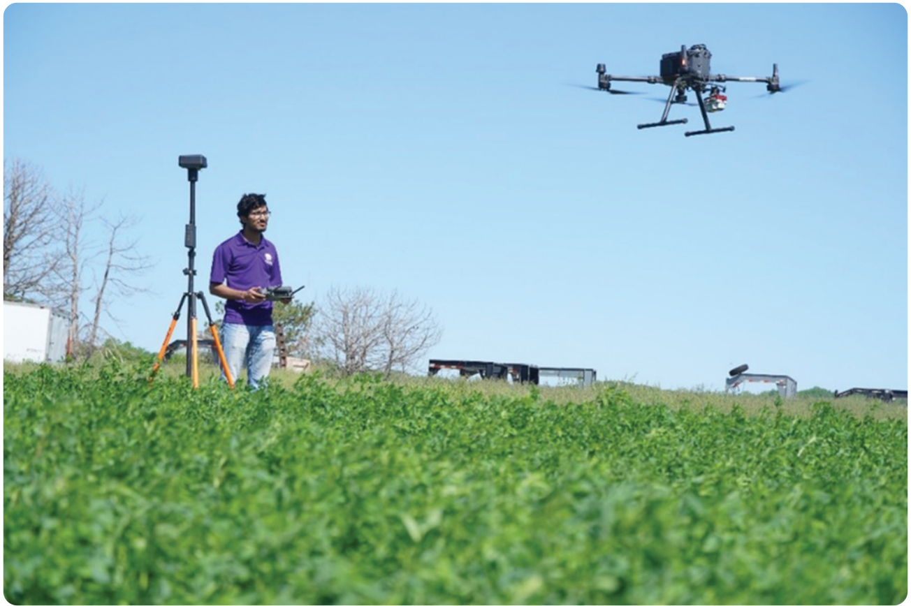
Figure 2. Collecting thermal and multispectral images of alfalfa.
