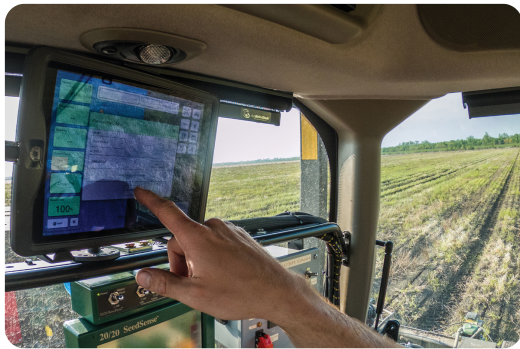
A farmer in a tractor/planter equipped with a planter monitor, a precision agriculture tool, to guide seed planting. Photo by Lance Cheung, USDA.
