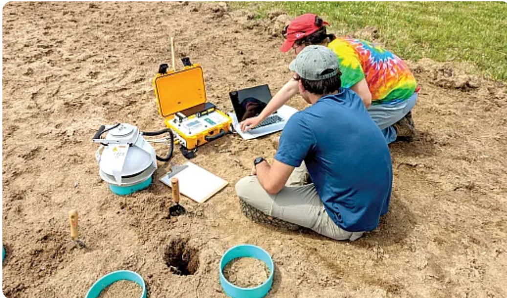
University of Tennessee Ph.D. students Kyle Brown (front) and Alexis Gillmore use an infrared gas analyzer to measure soil respiration in field sites as part of their research on degradation rates of biodegradable mulch. Photo by Morgan Isaacs.
