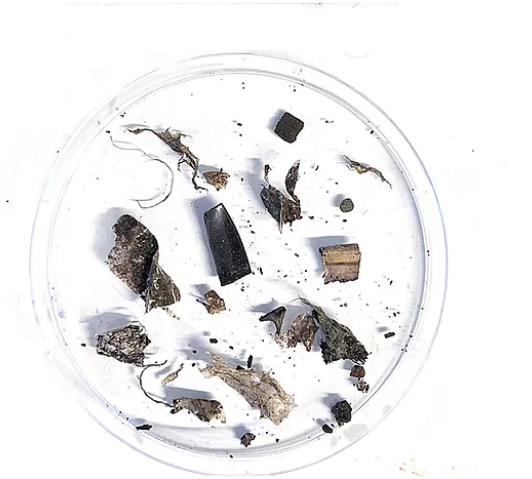
Anahita Khosravi, a Ph.D. student at the University of Massachusetts Amherst, first removed macroplastics from samples of organic fertilizer before analyzing them for microplastics. Pictured here are macroplastics she extracted from just 50 grams of compost. Photo by Anahita Khosravi.
