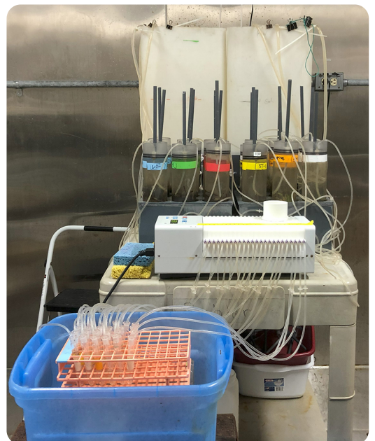
Sediment cores and site water arranged for continuous flow-through incubation experiments.
